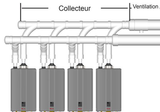
Figure 50: Installation de circuit commun d'évacuation PVC/CPVC
